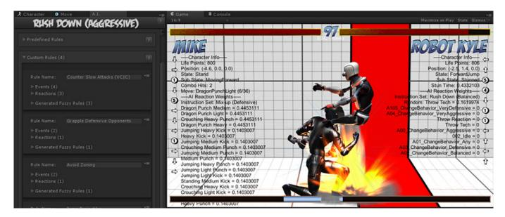
This add-on uses Fuzzy Logic to evaluate the information of the scene and calculate the desirability of each given action, translating the AI decisions directly into user input. In other words: the AI doesn't cheat, it uses the same input system used by the player.
