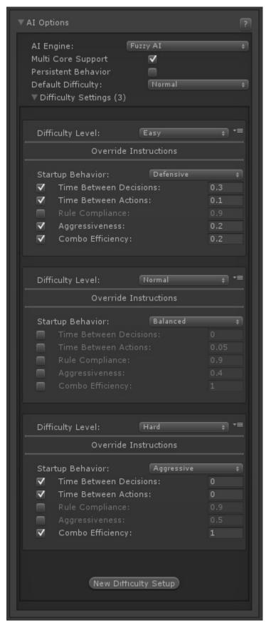
**Multi Core Support:** Tells UFE to run decision making process in its own thread. Multicore reduces CPU usage significantly, but makes the weight calculation slightly slower. Multicore puts the weight calculation into the Update() function, which makes the CPU run the process separately.
