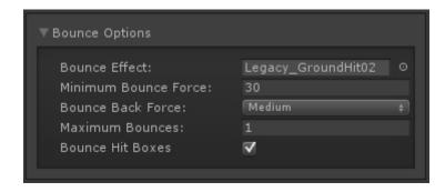
**Bounce Effect:** A prefab with particle effects that is fired when the character bounces of the ground.
